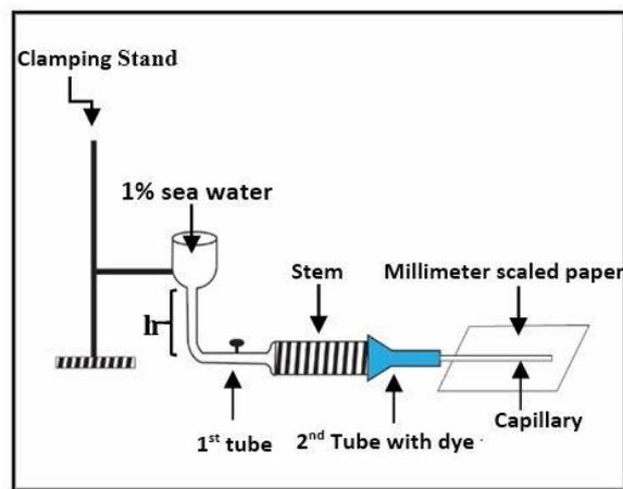
**Fig.2 Diagrammatic illustration of the manually designed Choatometer used in the experiment** [adopted from Choat *et al.* 2005] (“h” = height of the pressure head).
